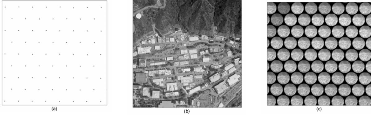
Figure 1. (a) A point source spot-image of a Shark-Hartmann sensor. (b) An object scene image used to create an SH extended-scene image for this study. (c) The SH extended-scene created by convolving (a) with (b).
